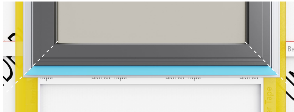
FIGURE 28. ALIGN CAP FLASHING MITRE CUTS WITH JOINERY MITRES
