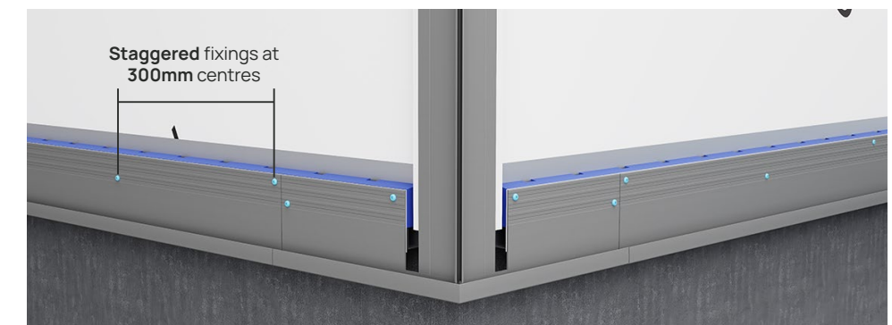
FIGURE 13. BASE CHANNEL FIXING
